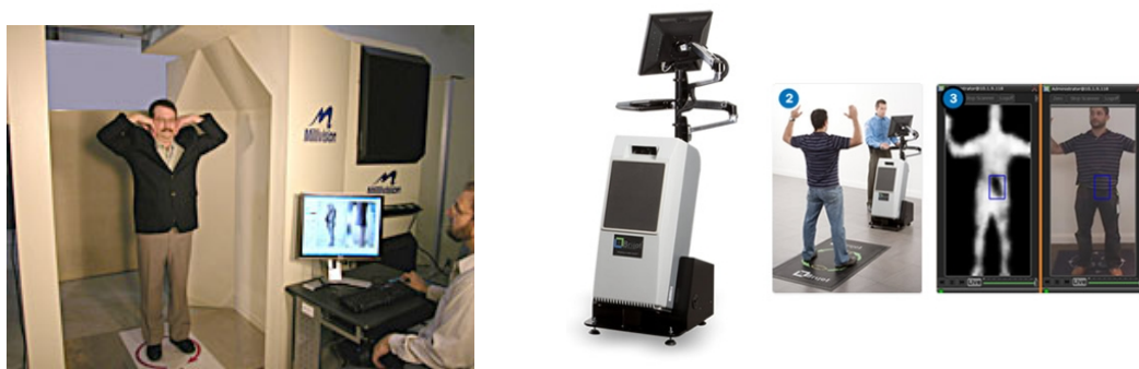
Fig.7 Passive Millimetre Wave Scanner and Image
