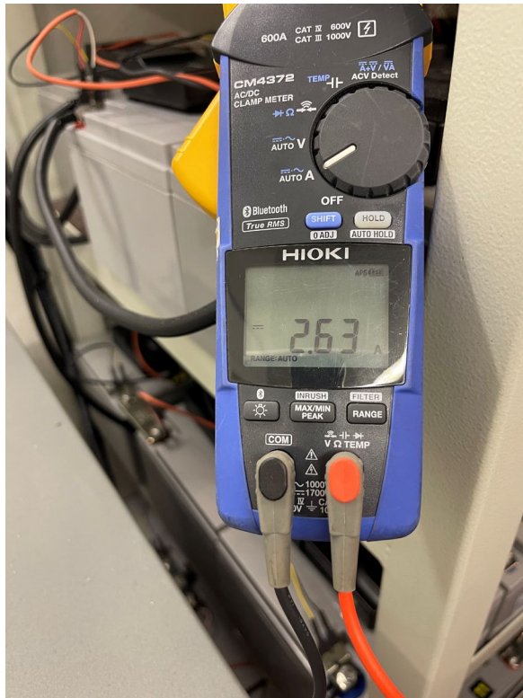
Battery charging current after dummy load test
